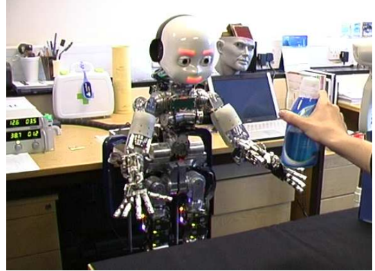
Fig. 3. iCub, the humanoid robot used in the experiments observing object-specific handling sequences by human demonstration.
